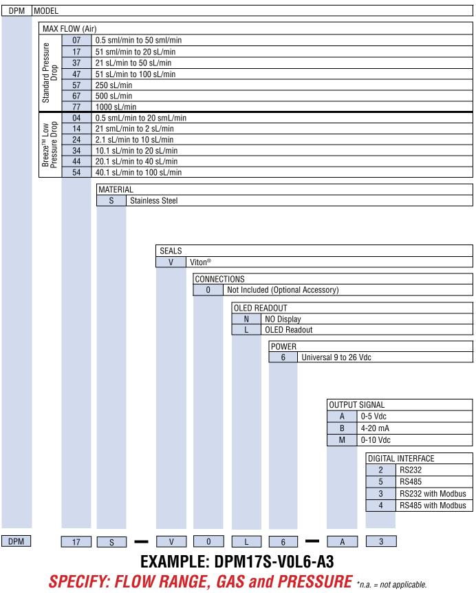
DPM17, 316 stainless steel, Viton® seals, with OLED readout 9-26 Vdc, 0-5 Vdc output signal,RS 232 with Modbus
