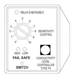
the probe, electrode wetting, and viscous liquids such as sludge. This close switching differential also allows the high electrodes to ignore foam layers. (Fixed sensitivity controllers without a close switching differential are only suitable for clean water applications).
