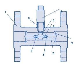
Housing 316 Stainless Steel Bearing Hanger 2 316 Stainless Steel 431 Stainless Steel 3 Rotor Spindle Tungsten Carbide PTFE/Carbon filled Bearing Bushes or Tungsten Carbide Thrust Ball Tungsten Carbide Pick off coil Stainless Steel body Collar 316 Stainless Steel
