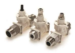
This multi-range radial flow turbine meter uses a low inertia turbine supported on robust sapphire bearings in a chemically resistant housing. Nine flow ranges (0.05 to 160 L/min), a choice of "plug in" fittings and individual traceable calibration make this meter one of the most flexible available.
