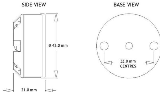
Mounting holes: two holes 5.5 mm diameter,
